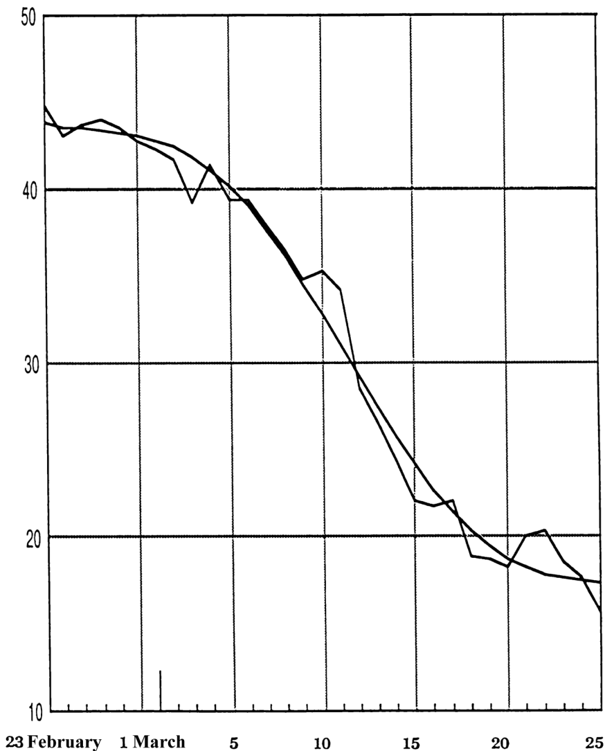
I.G.N. HALF-SUM (N+S)/2 OF THE AZIMUTHS OF THE SIGHTINGS AT MARKS Daily Averages 23 February - 25 March 1959 (31 days) in centesimal seconds counted positively in the clockwise sense Fitting to the sidereal period of the Moon of 27.322 days, with a linear trend
