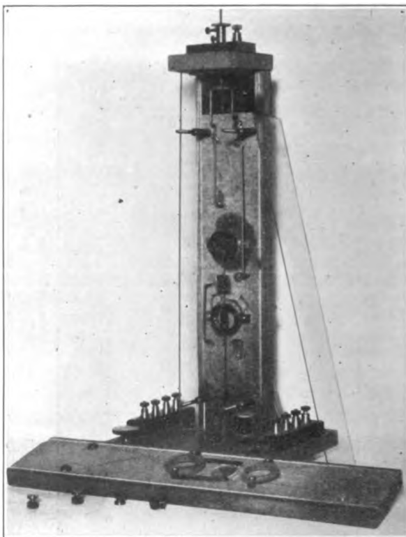
FIG. 2. Interior view of first meter
