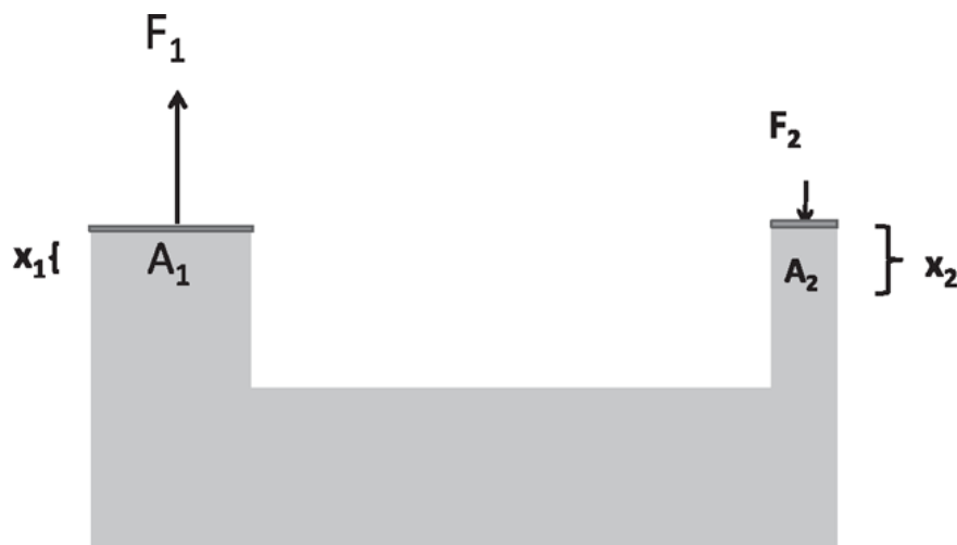
Figure 20.5 A hydraulic press that amplifies the force is made of two cylinders of different cross-sectional areas A_1 and A_2 , connected by a horizontal segment. Given P_2 = \frac{F_2}{A_2} = \frac{F_1}{A_1} = P_1 , the equality of the pressures, and A_1x_1 = A_2x_2 (the equality of volumes displaced in the two sides), we find \frac{F_2}{F_1} = \frac{A_1}{A_2} = \frac{x_1}{x_2} . A small force F_2 acting on the right cylinder pushes the incompressible fluid by a distance x_2 , and this leads to large force F_1 on the left that moves the piston over a smaller distance x_1 . Energy is conserved because F_1x_1 = F_2x_2 , as in a lever.
