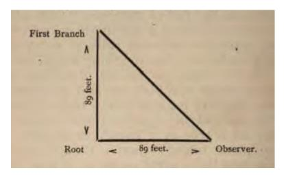
The reader will notice that the angle at the first branch is one of 45°, and the angle at the observer being the same, the *baseline and vertical must be the same length* AND CANNOT BY ANY POSSIBILITY BE LESS OR MORE. Therefore if we can get a position 45° north or south of the equator when the sun has no declination, the distance from our place of observation to the equator (the base of the triangle), will be exactly equal to the distance of the sun from the earth's equator (the vertical).
