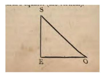
Let S E O be a right angled triangle, right angled at E; S the sun, E the equator, and O an observer at 45° north latitude.
