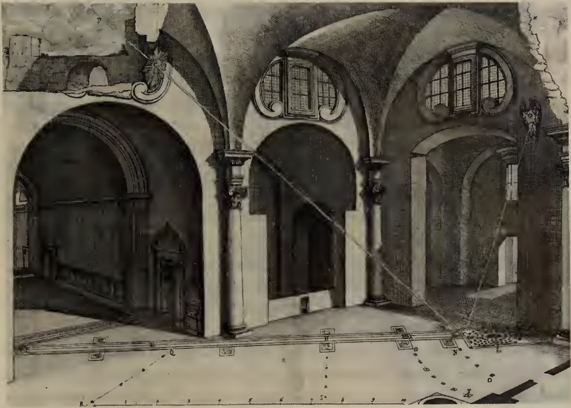
FIG. 5.2. The meridiana in S. M. degli Angeli, Rome. The ray from the right comes from the sun; that from the left, from a star near Polaris. From Bianchini, De nummo (1703).
