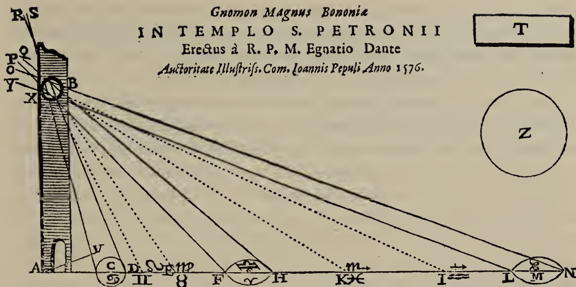
FIG. 2.31. Danti's meridiana in San Petronio. T is the cross-section, Z the size and shape of the hole. From Riccioli, Almagestum novum , 1:1 (1651), 132.
