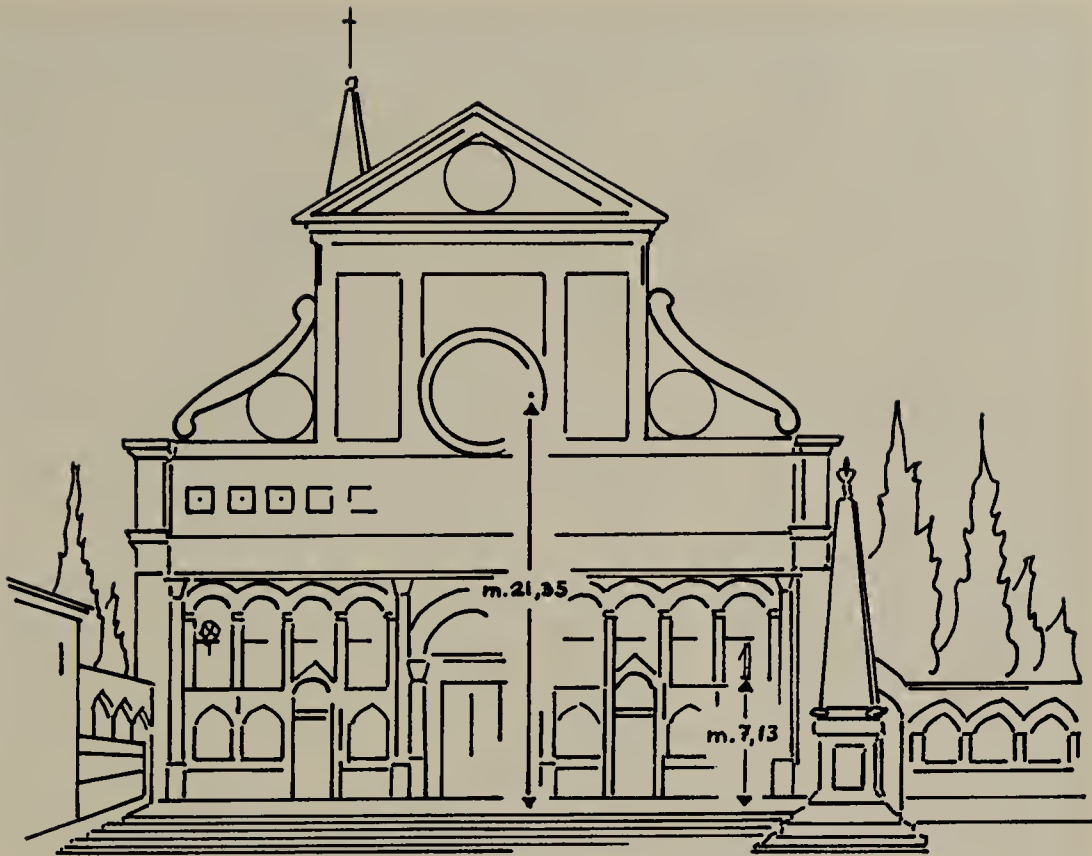
FIG. 2.28. Sketch of the façade of S. M. Novella, Florence, showing the placements of Danti's armillary, quadrant, and gnomon. From Righini-Bonelli and Settle, IMSS, Annali , 4:2 (1979).
